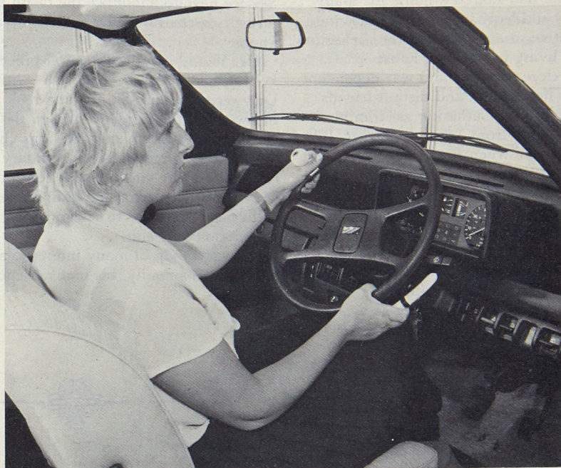
Illustrated above is the well-known Ashley Mobility Single Lever Brake & Throttle Hand Control Conversion for disabled drivers. The Control operates in the same 'plane' and shown above is an upward movement for accelerating. For braking, the Control is moved downwards.
